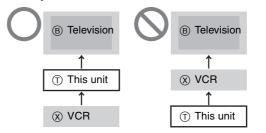
•When connecting to a television with a built in VCR, connect to the input terminals on the television side, not the VCR side.
