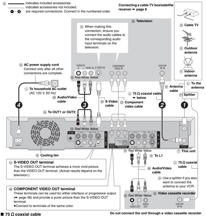
The picture and sound signal from this unit does not go through the 75  $\Omega$  coaxial cable to the television. Make sure you connect one of the following terminals on this unit to the television: the AUDIO/ VIDEO OUT terminal, the S-VIDEO OUT terminal or the COMPONENT VIDEO OUT terminal. If the television has none of
